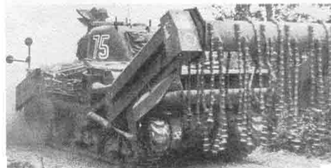
A Sherman "Crab". The chains were used to explode mines by flailing.
